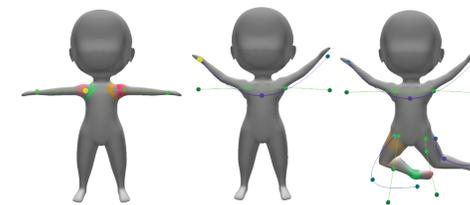
Baseline strokes select joints, and offset strokes define the desired pose. Bones are rotated and optionally stretched to best match the pose. To refine the pose, the user can adjust control knots on the strokes or draw new ones.
