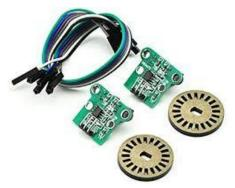
A ROTARY ENCODER IS A TYPE OF POSITION SENSOR WHICH IS USED FOR DETERMINING THE ANGULAR POSITION OF A ROTATING SHAFT. IT GENERATES AN ELECTRICAL SIGNAL, EITHER ANALOG OR DIGITAL, ACCORDING TO THE ROTATIONAL MOVEMENT.
