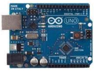
THE **ARDUINO UNO** IS A MICROCONTROLLER BOARD BASED ON THE ATMEGA328. IT HAS 20 DIGITAL INPUT/OUTPUT PINS (OF WHICH & CAN BE **USED** AS PWM OUTPUTS AND & CAN BE **USED** AS ANALOG INPUTS), A 16 MH2 RESONATOR, A USB CONNECTION, A POWER JACK, AN IN-CIRCUIT SYSTEM PROGRAMMING (ICSP) HEADER, AND A RESET BUTTON.
