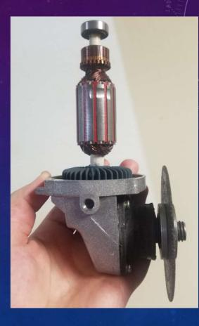
• Removed windings, weights, fan, and insulation
